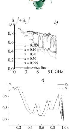
Figure 3: Relationship of losses (absorption) of microwave energy in the strip line without specimens (continuous lines) and with the specimens (dotted lines and dash-dot lines) of SS systems (1-x)NaNbO<sub>3</sub>-xCa<sub>2</sub>Nb<sub>2</sub>O<sub>7</sub>) (*a*), (1-x)NaNbO<sub>3</sub> - xSr<sub>2</sub>Nb<sub>2</sub>O<sub>7</sub> (*b*), Relationships of losses (absorption) of microwave energy of SS of the studied systems (c).
