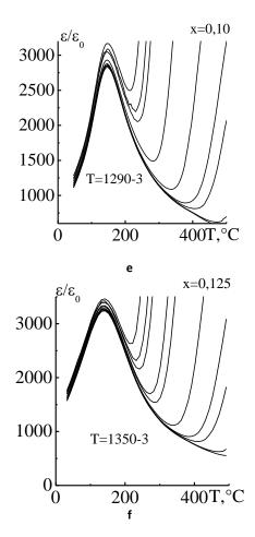
Figure 7: Temperature relationships of dielectric permeability ( $\epsilon/\epsilon_0$ ) of the studied object for various contents of Ca<sub>2</sub>Nb<sub>2</sub>O<sub>7</sub> – (a, b, c) and Sr<sub>2</sub>Nb<sub>2</sub>O<sub>7</sub> – (d, e, f).
