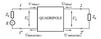
Figure 1: Scheme demonstrating connection of the quadripole in long transmission line.
