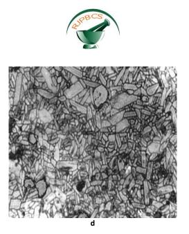
Figure 5: Transitions of microstructure of SS  $(1-x)NaNbO_3 - xCa_2Nb_2O_7$ ). In Figures x = 0 (a), x = 0.20 (b), x = 0.70 (c), x = 1.0 (d). Magnification x300.
