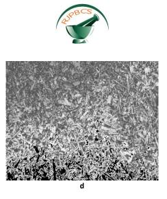
Figure 6: Transitions of microstructure of SS  $(1-x)NaNbO_3 - xSr_2Nb_2O_7$ ). In Figures x = 0.075 (a), x = 0.20 (b), x = 0.80 (c), x = 1.0 (d). Magnification x300.
